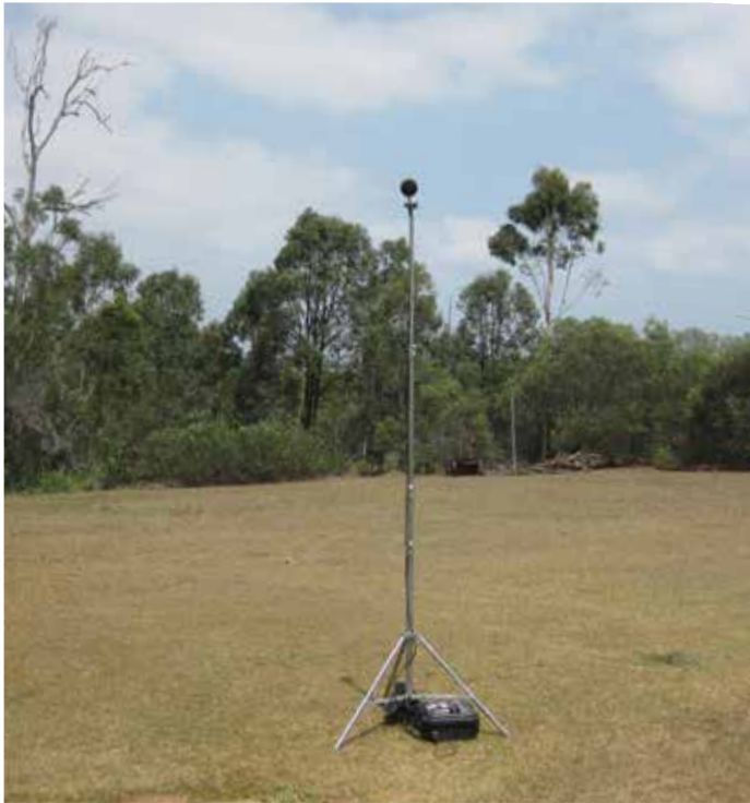
The operational noise assessment involved placing free standing noise monitoring devices (and sometimes a weather station) at identified properties for several days.
