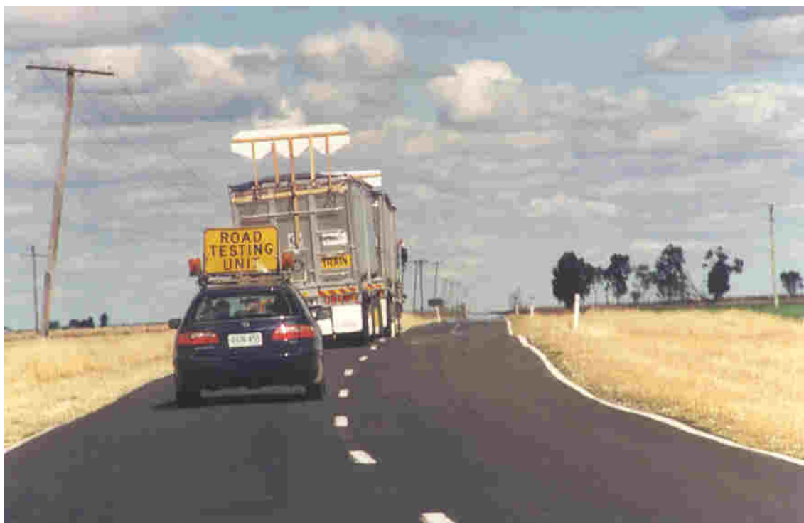
Figure 4.27 Testing the tracking characteristics of a MCV on a rough surface and narrow formation with 3m to 3.5m lanes (Haldane, 2002)
