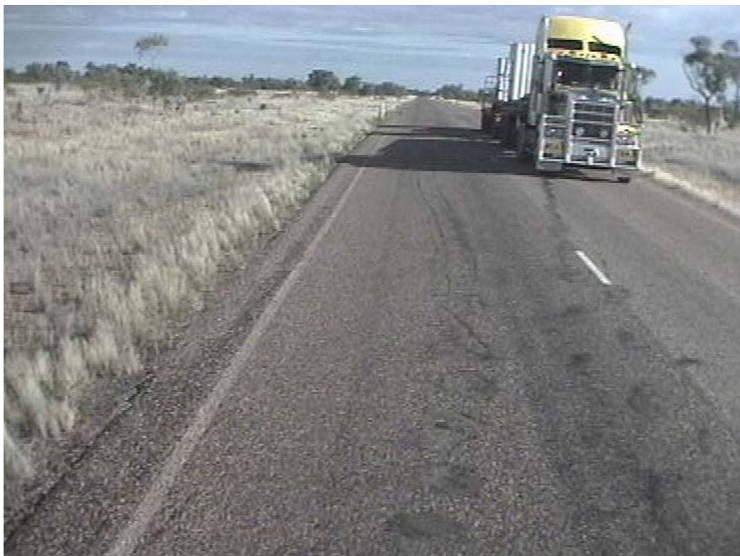
Figure 4.25 Example of Type 2 road train operating on a 7.9m carriageway with full width seal on a low formation
